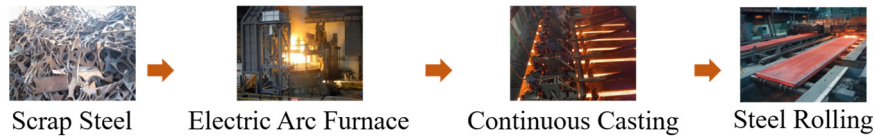
Figure 2. Schematic diagram of short-process steelmaking.
