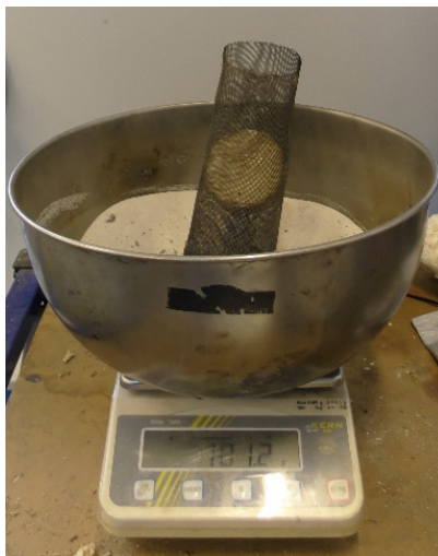
Figure 4. Sample weighing during a burning rate experiment.
