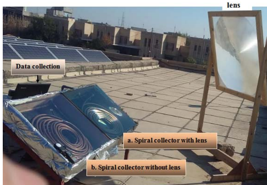
Figure 1. Solar system a) spiral without lens b) spiral with lens.
