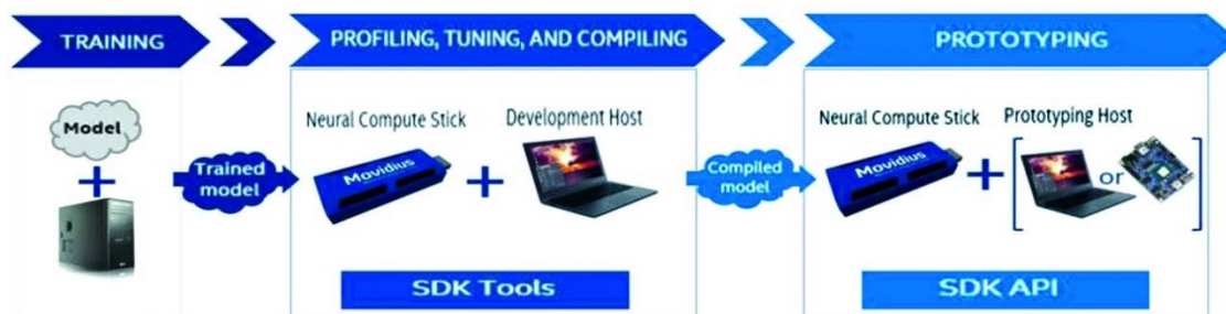
Figure 5. The development process of the NCS is presented in the workflow diagram.
