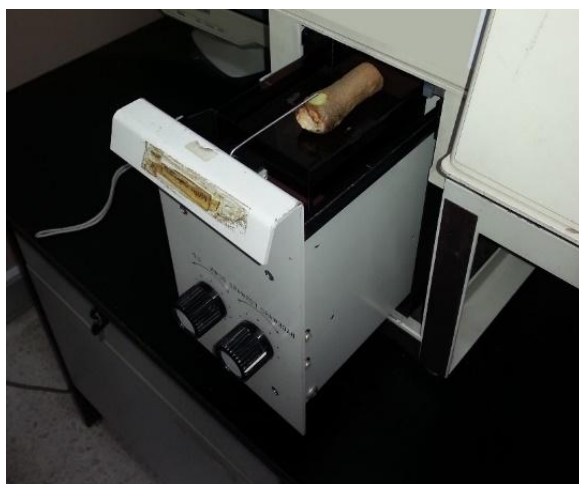
Figure 2. Placement of the durian stem, separated from the fruit, in the sample drawer of the spectrometer.
