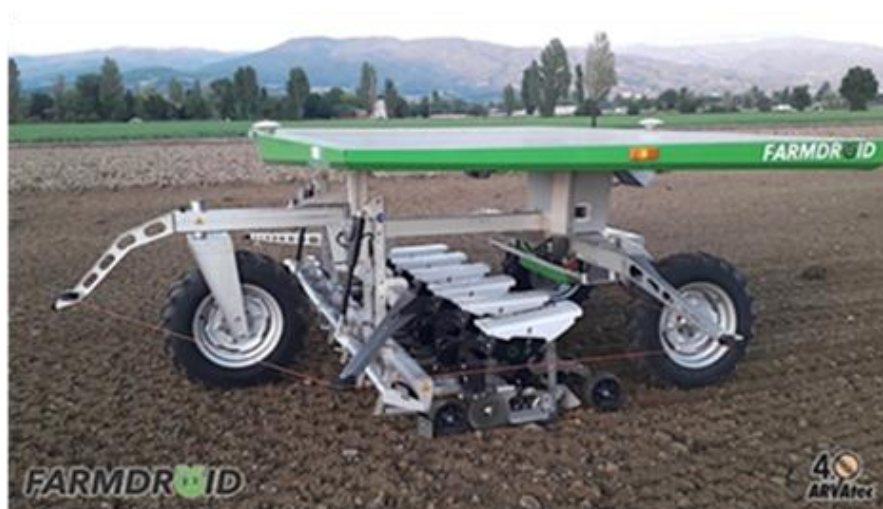
Figure 6. Field robot FarmDroid FD20 for precision seeding and herbicide spraying (ARVAtec) [44].
