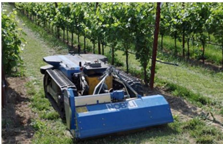
Figure 16. Robot Hammerhead FR-01 developed by the startup Field Robotics for vineyard crop operations [73].
