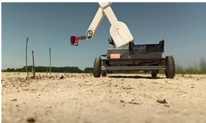
Figure 11. Robot Gus of Autopickr for asparagus harvest [68].
