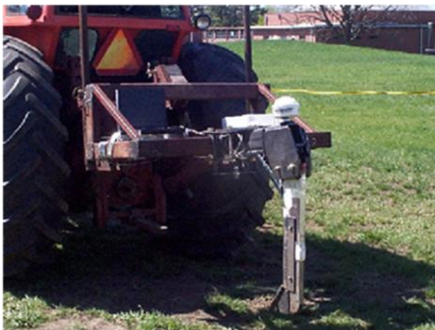
Figure 2. System for setting up the working depth of a ripper to perform spatially variable soil tillage.
