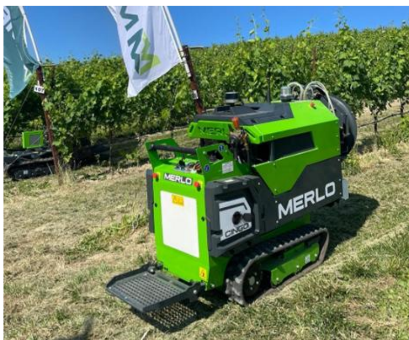
Figure 9. Tracked unmanned electrical transporter Merlo Cingo M600A-e that converts into a sprayer for vineyards [52].
