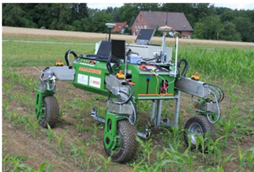
Figure 19. BoniRob robot, developed by Amazone-Werke, in association with Robert Bosch GmbH, Osnabrück University of Applied Sciences and other partners [76].
