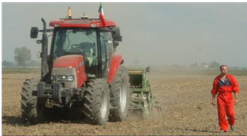
Figure 5. An unmanned tractor is an agricultural machine equipped with an automatic guidance system, enabling the farmer to accurately follow previously planned trajectories in a field.
