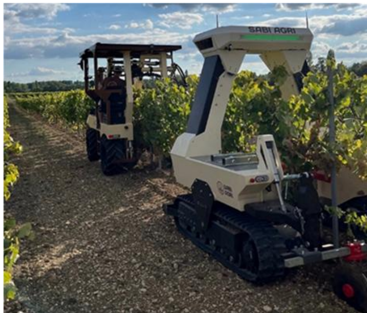
Figure 20. Electrical overstepping tractor Alpo (left) and electrical overstepping robot Zilus (right) of Sabi Agri for carrying out crop operations in synergy in a vineyard (here) or another fruit tree orchard [77].
