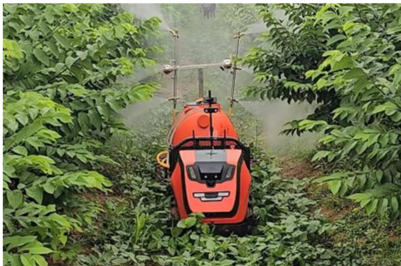
Figure 21. Electrical robot iMog of Farmrobo Technologies during spraying by means of a mist blower [78].
