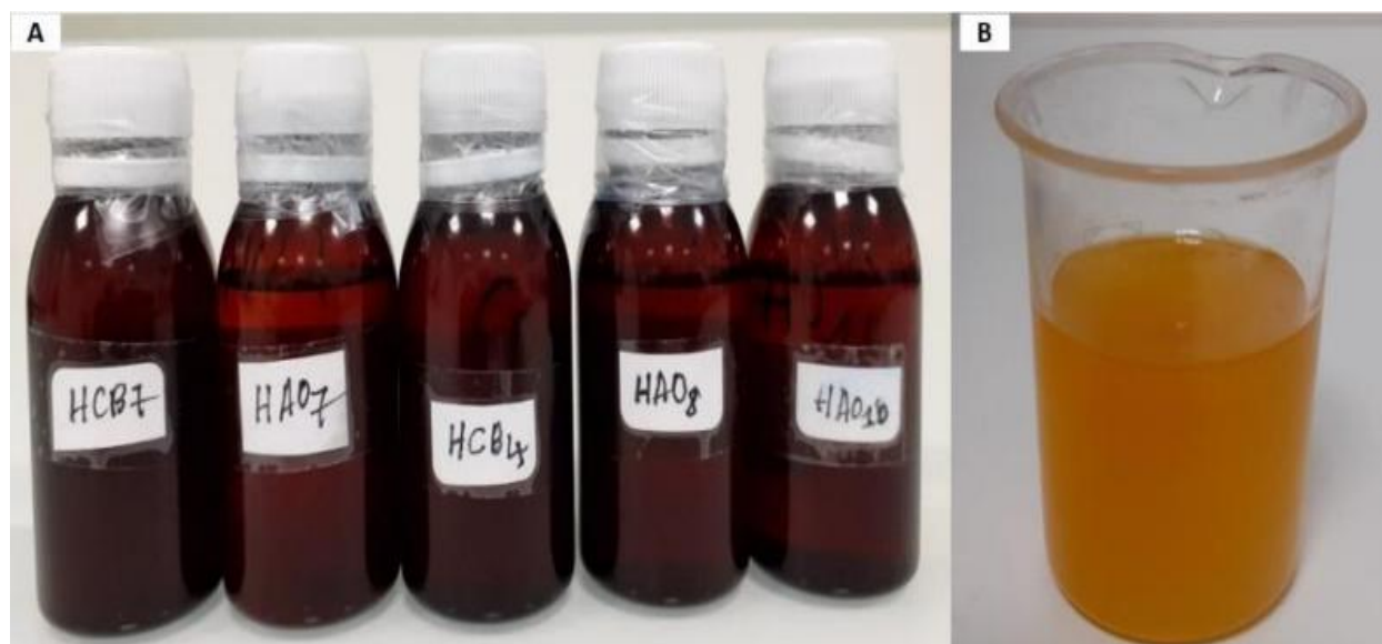
Figure 1. Oil samples after opening for analysis; A: HCB: Cottonseed oil collected in Bobo Dioulasso; HAO: Peanut oil collected in Ouagadougou; Numbers 4, 7, 8 and 10 are the samples numbers. B: Crude peanut oil in a beaker.
