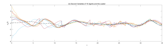
(b) Synchronization results with 4 pinned nodes in the second layer.
