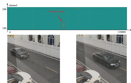
Figure 3. Data acquisition scheme of Traffic vibration signal. On the left is a diagram of the data acquisition scheme, and on the right is the actual fiber laying circuit diagram.
