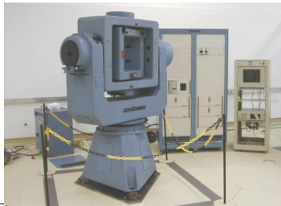
Figure 11. Three-Axes motion simulator (CETT-CONAE).
