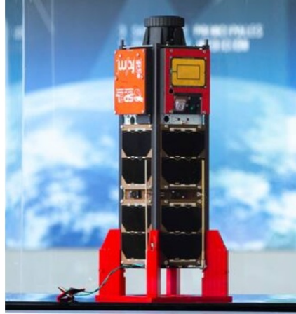
Figure 3. 3U PlantSat, part of the SUCHAI swarm of CubeSats developed by Universidad de Chile.
