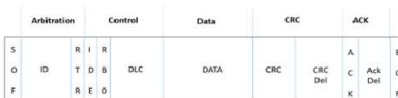
Figure 4. The structure of a CAN data frame.
