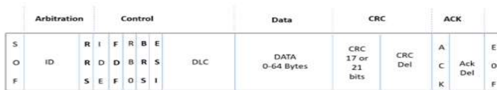
Figure 5. The structure of a CAN FD data frame.
