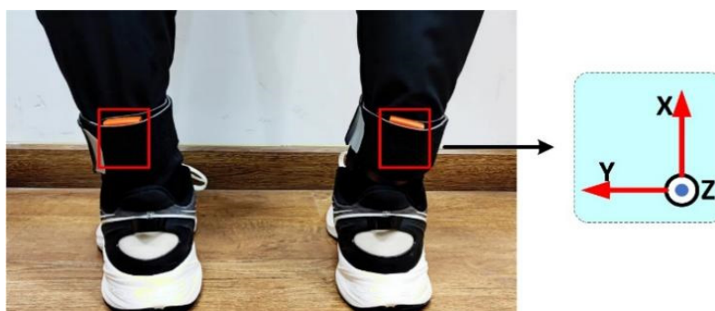
Figure 2. Wearable Xsens sensor installation.
