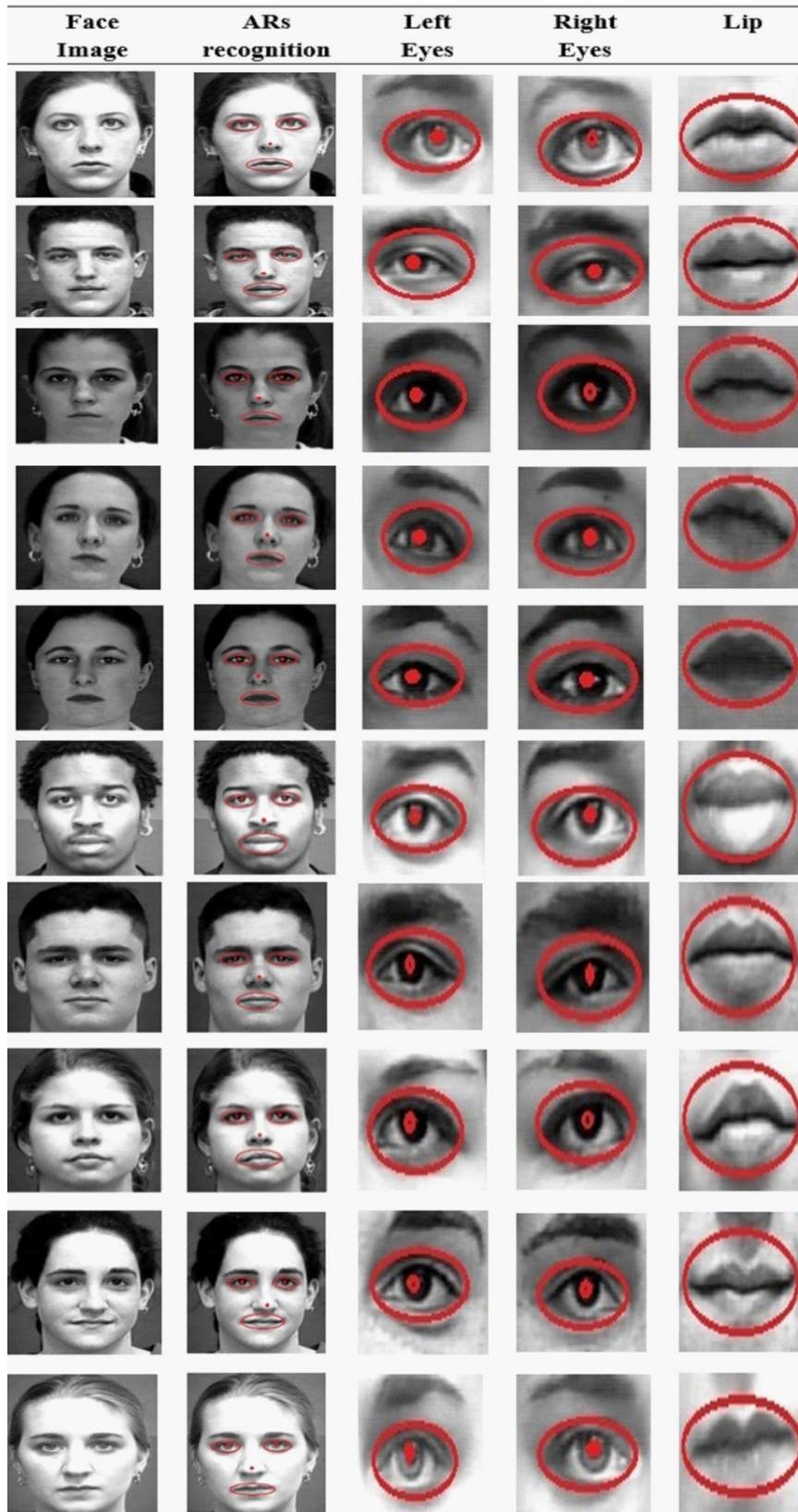
Figure 6. Original images are in column-1. Images after regions detection are in column-2. Column-3 show left eyes detection. Fourth column shows right eyes detection and fifth column shows lip region detection.
