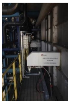
Figure 2. Measurement of the outer-surface temperature using a multispectral probe.
