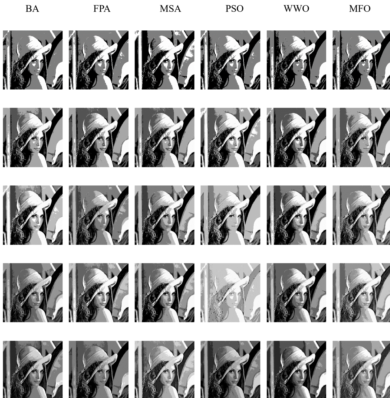
Figure 5. Segmentated images of Test 1 for different algorithms using Kapur method at levels 2, 3, 4, 5 and 6.
