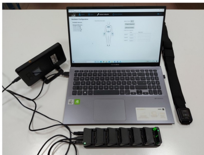
Figure 1. Opal System: Mobility Lab Software, Access Point, Docking Station, a movement monitor. Modified with permission from Donisi et al. , Sensors; published by MDPI, 2021.
