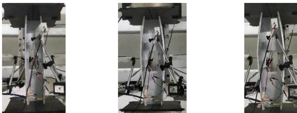
(a) Distortional buckling
