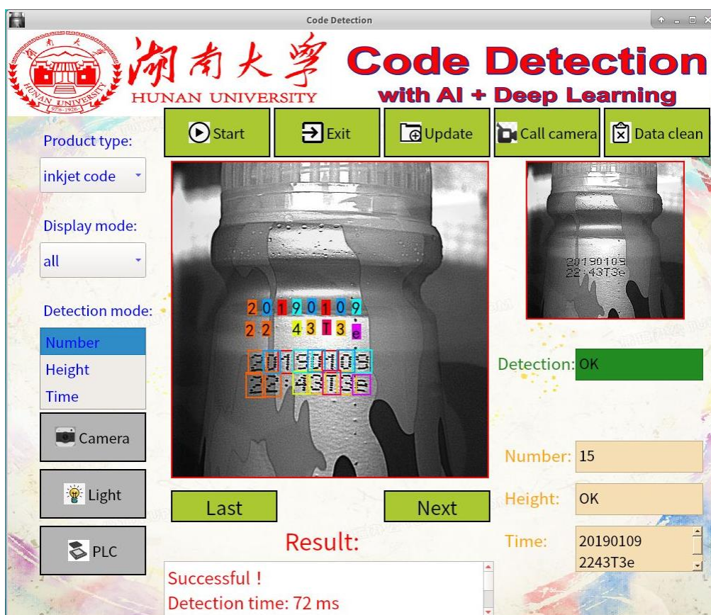
Figure 16. The interactive main interface of the code defect detection system.
