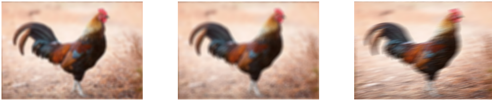
Figure 8. The original RGB image degraded by blurred matrices M_1 , M_2 and M_3 respectively.
