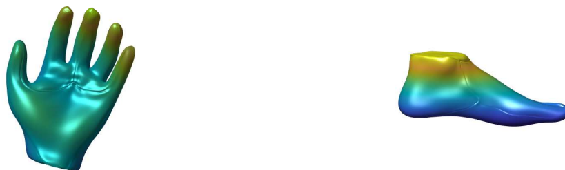
(a) A “human hand” solid model defined by a 3D Bézier volume. (b) A “human foot” solid model defined by a 3D Bézier volume.
