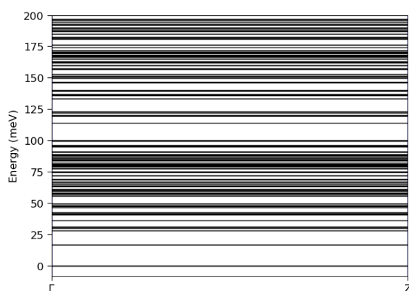
Figure 5. Phonon band structure for C_{60}Si .
