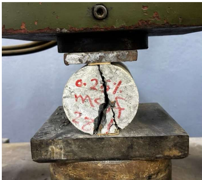
Figure 6. Splitting tensile strength test for SCC reinforced with 0.25% HMSF.
