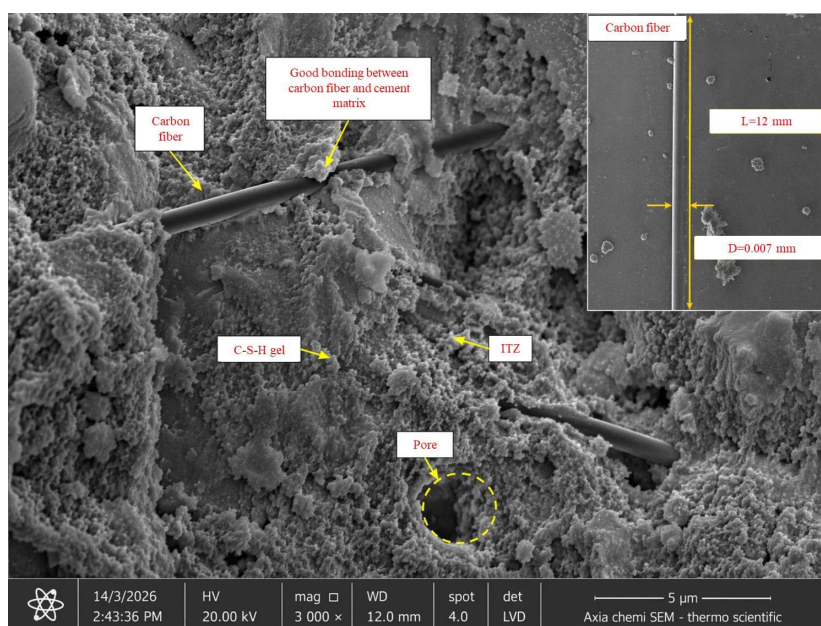
Figure 11. SEM image for SCC reinforced by CCF at 4000 \times .
