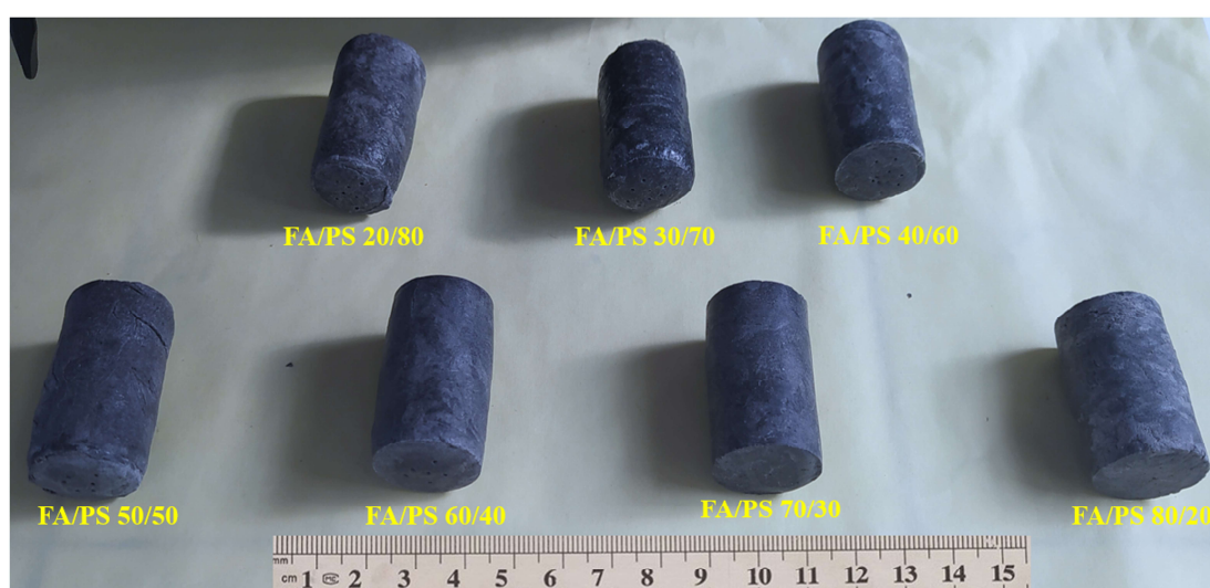
Figure 4. Macroscopic appearance of elaborated FA-PS composites with varying fly ash/polystyrene ratios (20/80 to 80/20).
