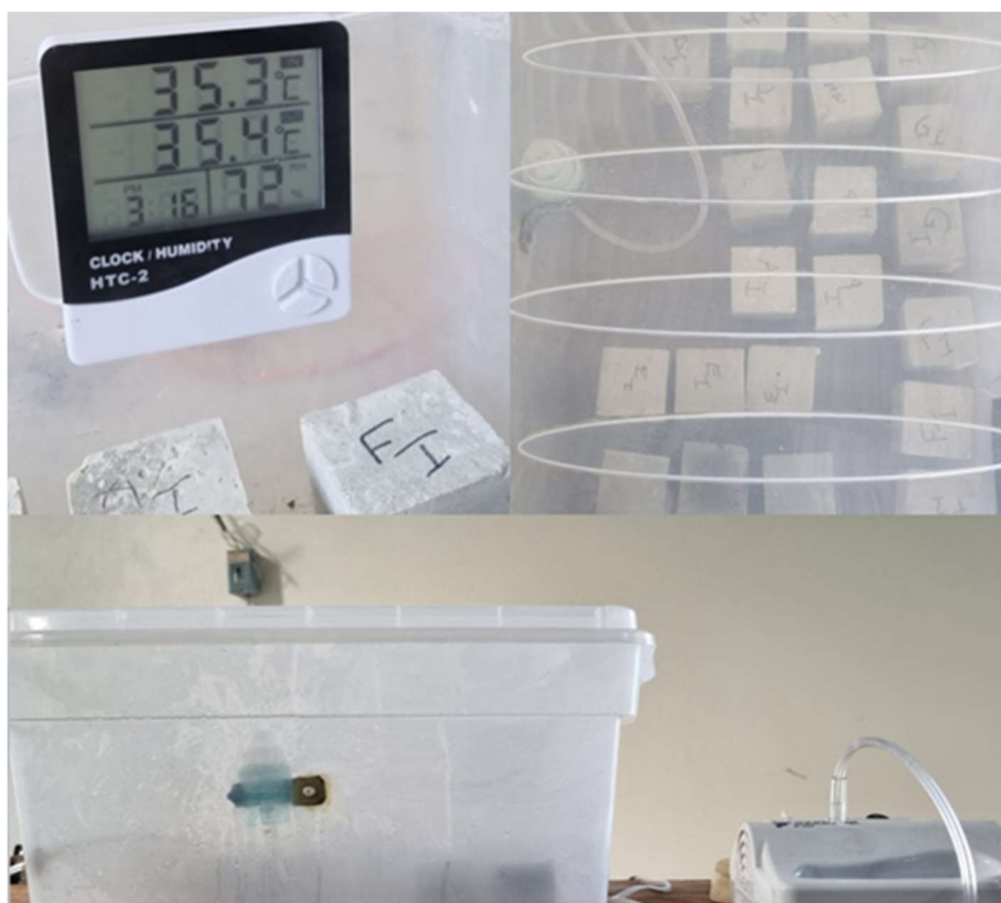
Figure 5. Exposure of samples to accelerated marine breeze conditions.
