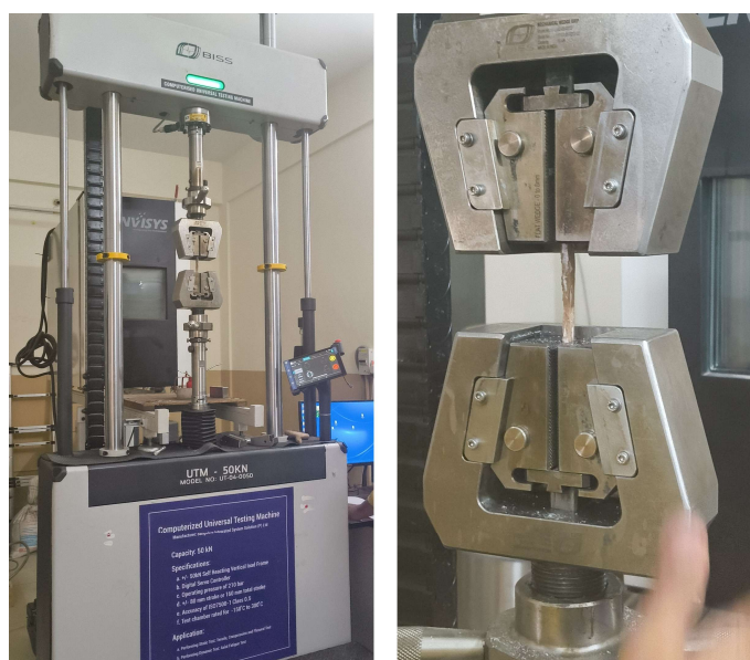
Figure 3. Tensile properties testing of composite specimens using UTM.
