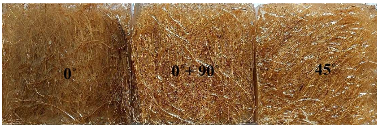
Figure 1. Epoxy composites reinforced with coir in 0, 0 + 90, and 45° orientations.
