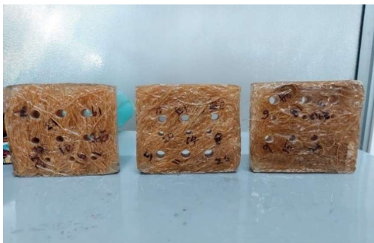
Figure 8. Composite materials after drilling operation.
