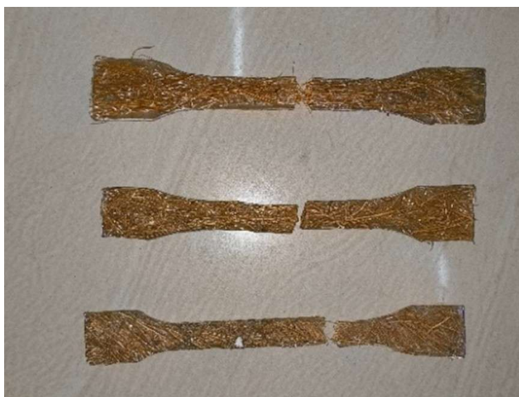
Figure 7. Composite specimens after tensile test.
