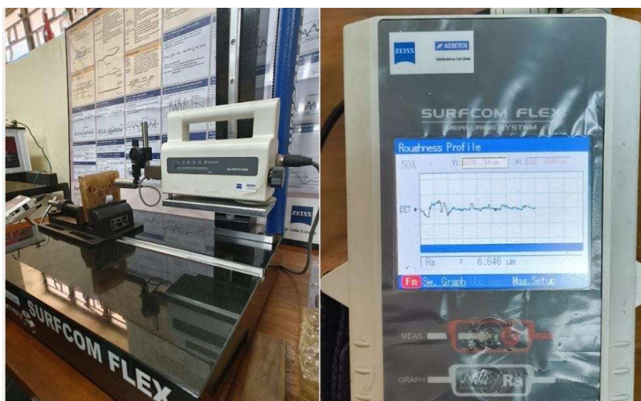
Figure 5. Measurement of Ra using the Surfcom Flex 50-A.
