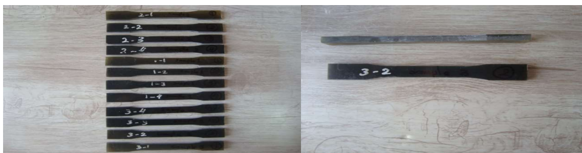
Figure 2. Standard tensile test specimens.
