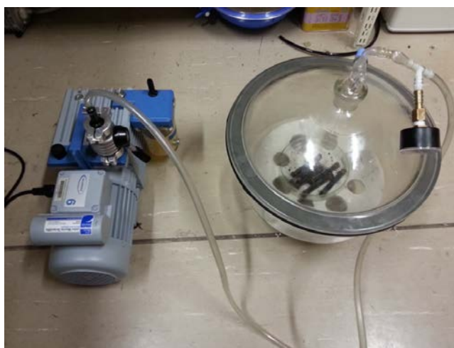
Figure 1. The set-up used for vacuum assisted vapor phase polymerization with EDOT:THF solution.
