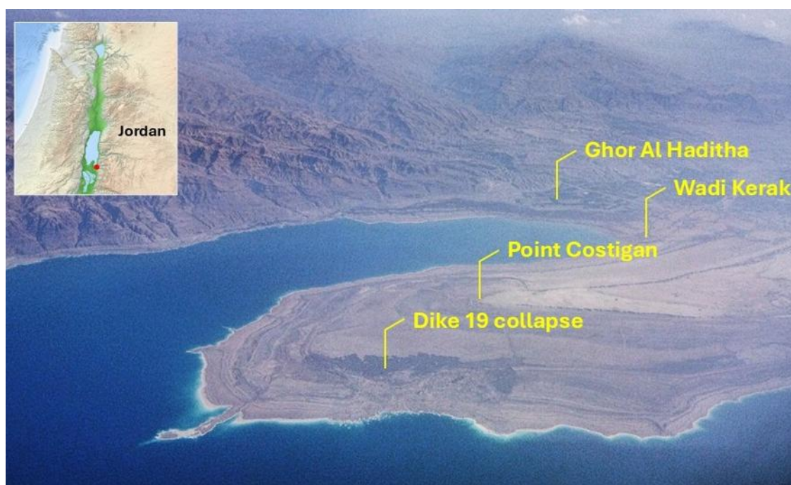
Figure 1. Eastward-looking aerial view of the Lisan Peninsula and Ghor Al-Haditha, Jordan, acquired in 2011. From the 1960s to 2026, the Dead Sea water level has declined by 46 m (from -395 \text{ m} to -441 \text{ m} ). As a result, a wave-cut platform, approximately 1.6 to 5 km in width, has developed around the former Point Costigan. The failure of Arab Potash Company's Dike 19 on 22 March 2000 exemplifies the geotechnical instability of this recently exposed terrain.
