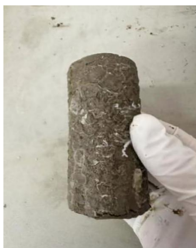
Four sulfuric acid erosion cycles
