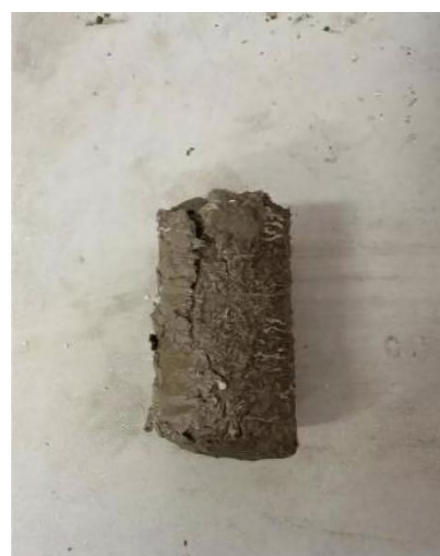
Six sulfuric acid erosion cycles
