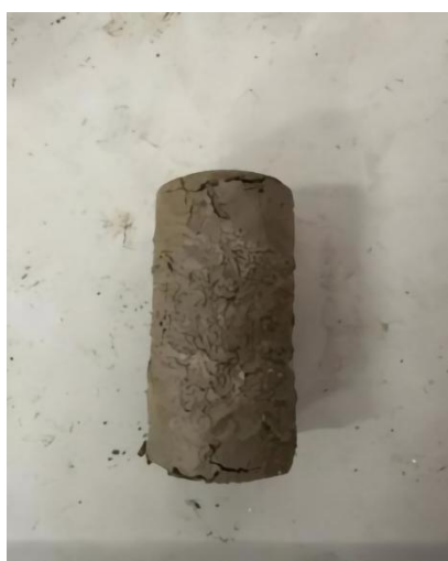
Two sulfuric acid erosion cycles
