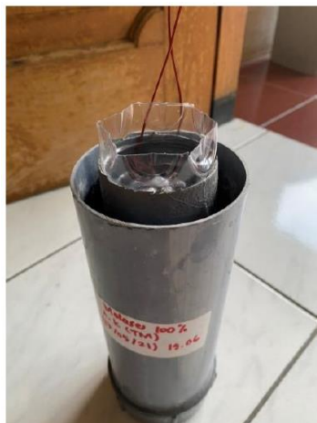
Figure 1. Prototype tubular microbial fuel cell.
