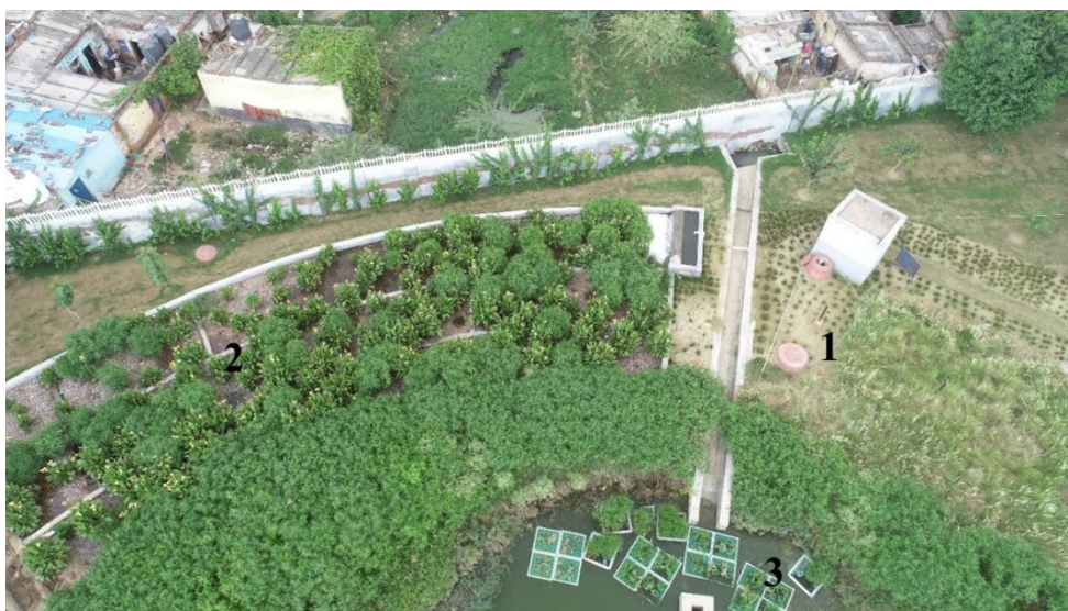
Figure 4. Aerial image of the SWAB system (1) Biodigester (2) Scientific Wetland and (3) Floating wetlands.
