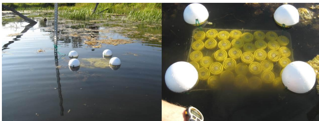
Figure 1. Randomized array of CES deployed in pond.
