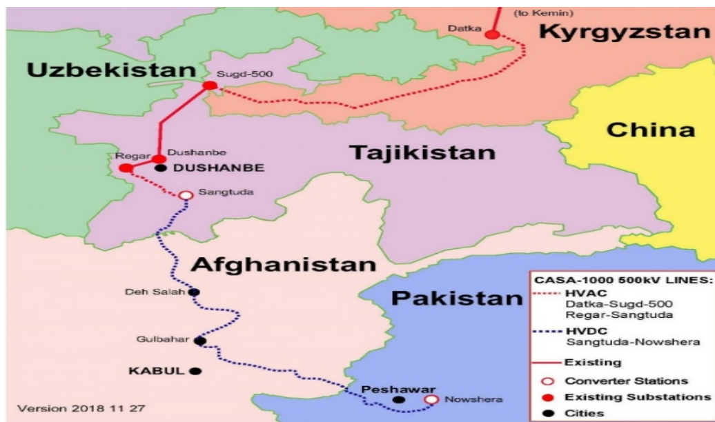
Figure S8. CASA-1000 transmission line. Source: [5].
