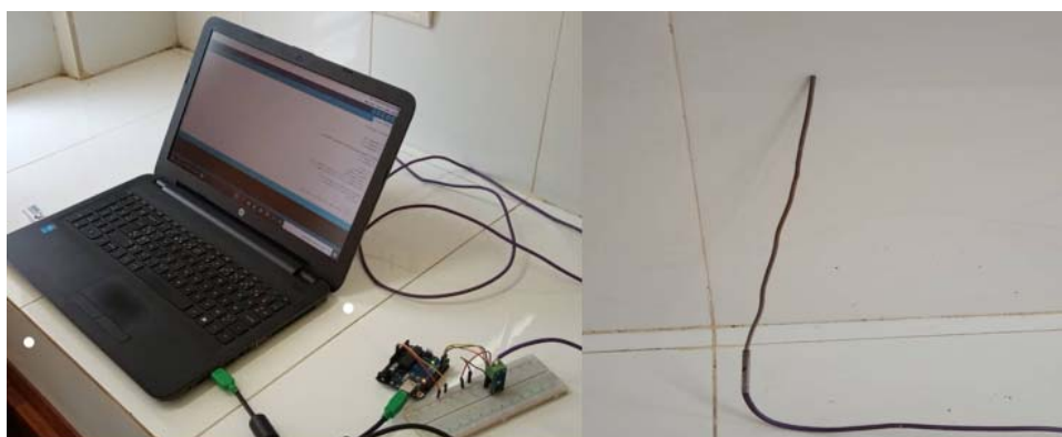
Figure 6. Data acquisition system + thermocouple.
