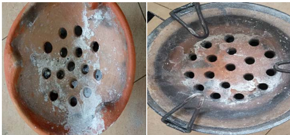
Figure 16. Clay (left) and Nansu (right) stoves after durability test.
