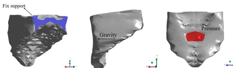
Figure 5. Soft palate boundary conditions. The loading surface (red) approximates the tensor veli palatini insertion, with pressure applied in the negative X-axis direction to simulate muscle tone opposing gravity.
