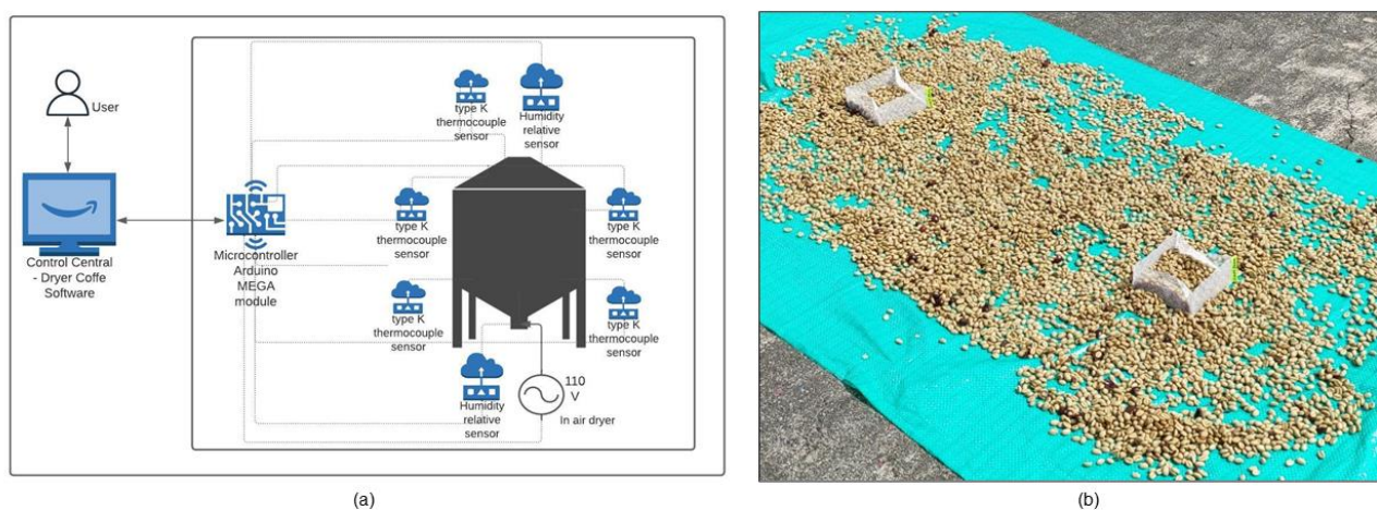
Figure 1. (a) Diagram of the equipment used for drying coffee with hot air and (b) open sun.
